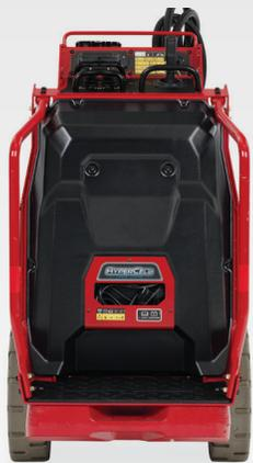
**30" Width** - The new, next generation eDingo has a brand-new frame with a narrow footprint to easily fit through a 3-ft. door
