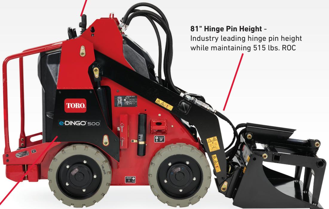
**81" Hinge Pin Height** - Industry leading hinge pin height while maintaining 515 lbs. ROC
