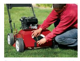
The seed flow rate can be adjusted on the fly for different applications and seed types.
