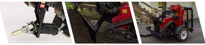
Simplify irrigation and cable installations under driveways and sidewalks with the bore drive head. It can be lowered into the trench to aid in level operation.
