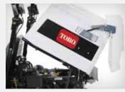
**HIGH CAPACITY** The 9.5-bushel hopper means less time emptying and more time mowing. Exclusive baffle design fills design handles taller grass and evenly back to front for maximum efficiency.
