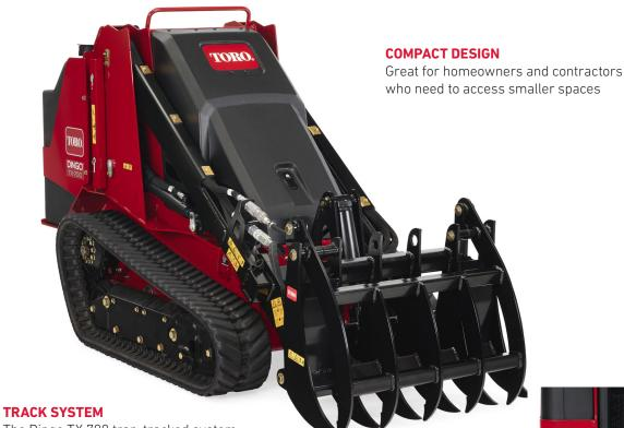
The Dingo TX 700 trap-tracked system, offers peace of mind and comes with either an aggresive narrow track or turf-friendly wide track option
