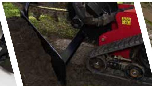
Backfill open trenches efficiently and finish the job with the backfill blade, which can be installed in less than a minute.
