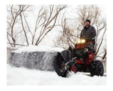
55" (139.7 cm) Power Broom is designed to tackle sidewalks and clear snow and debris down to the pavement.
