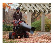
The Pro Force Blower has a 360° nozzle rotation and utilizes the MULTI FORCE 26.5 hp Kohler<sup>®</sup> Command Pro<sup>™</sup> EFI engine to deliver tremendous air power for fast removal of grass clippings, leaves, or other debris.
