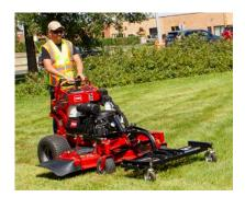
Turn your mower into the ultimate spring clean-up tool with MULTI FORCE frontmount tine rake dethatcher. Use the rake to remove thatch, embedded leaves and debris.
