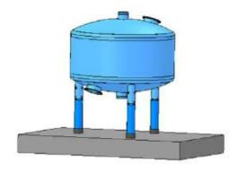
**Step 2** –Carefully raise the media filter (4) with \*\*quilted forklift or tilt it, and remove the rubber caps (6) from the
