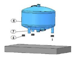
Step 4 – Attach the extension legs (2) to the media filter legs (7) either using a \*\*quilted forklift or by tilting
