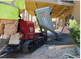
Built on the trusted tracked Ultra Buggy frame, the swivel buggy gives you a 180 degree dump radius, plus:
