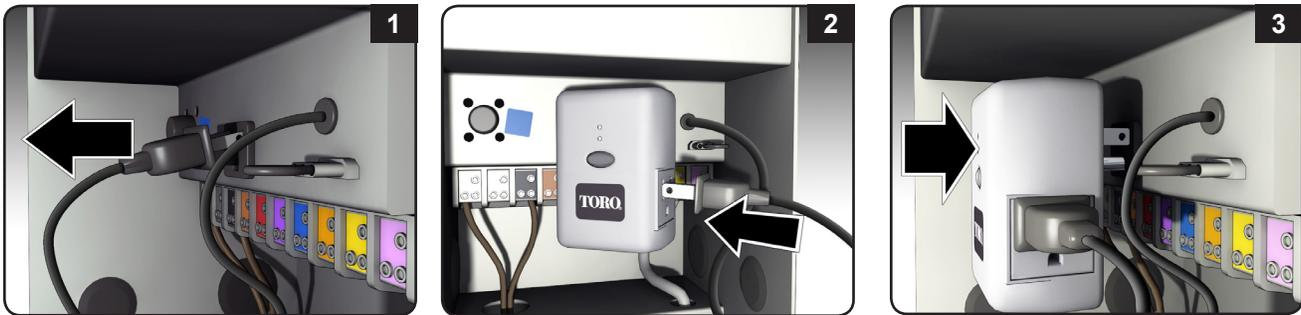
The EVO-AR works with any residential transformer with an internal AC outlet. One can also plug the AR unit directly into a wall outlet and then plug an electronic device into the AR's own outlet, such as holiday lights or a fountain.
